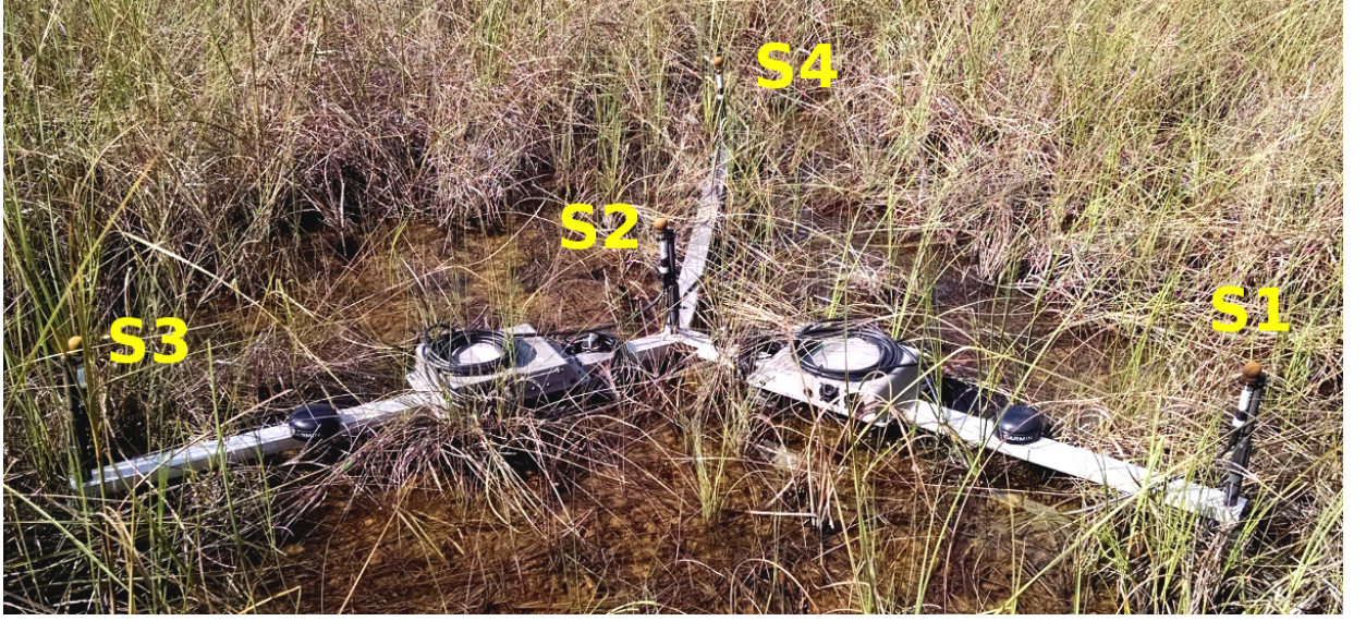
Figure 1. Acoustic array on July 8, 2016 consisting of (4) SMM-A1 microphones denoted S1, S2, S3 and S4, (2) SM3BAT digital recorders, and (2) SM3 GPS antenna. The S1 - S2 arm is aligned east - west. Sensor S1 is located at 25.33754^{\circ} N, 80.79918^{\circ} W.
